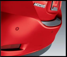
**REAR PARKING SENSORS\*** Mounted discretely within the lower bumper, the Rear Parking Sensors notify the driver of obstructions behind the vehicle using an alarm sound.
