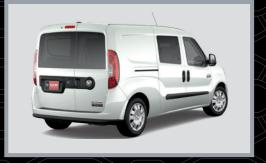
OFFSET DOORS DESIGNED TO BE SIMPLER AND SAFER. Positioning the larger of the two rear doors on the left gives you 10 percent greater access than typical 50/50 doors and lets you access the rear cargo area with greater confidence when traffic is adjacent. When the right side is open, there's less door width to move around.
