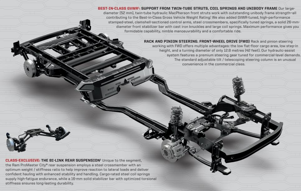
**FRAME STRENGTH** The body-frame integral (unibody) design includes an integrated frame, boxed frame components, multiple crossrails and a robust suspension. The engineering gives Cargo Van Best-in-Class payload up to 862 kg (1,900 lb), unsurpassed towing up to 907 kg (2,000 lb), Best-in-Class GVWR of 2,447 kg (5,395 lb) and a Gross Combined Weight Rating (GCWR) of 2,676 kg (5,900 lb).
