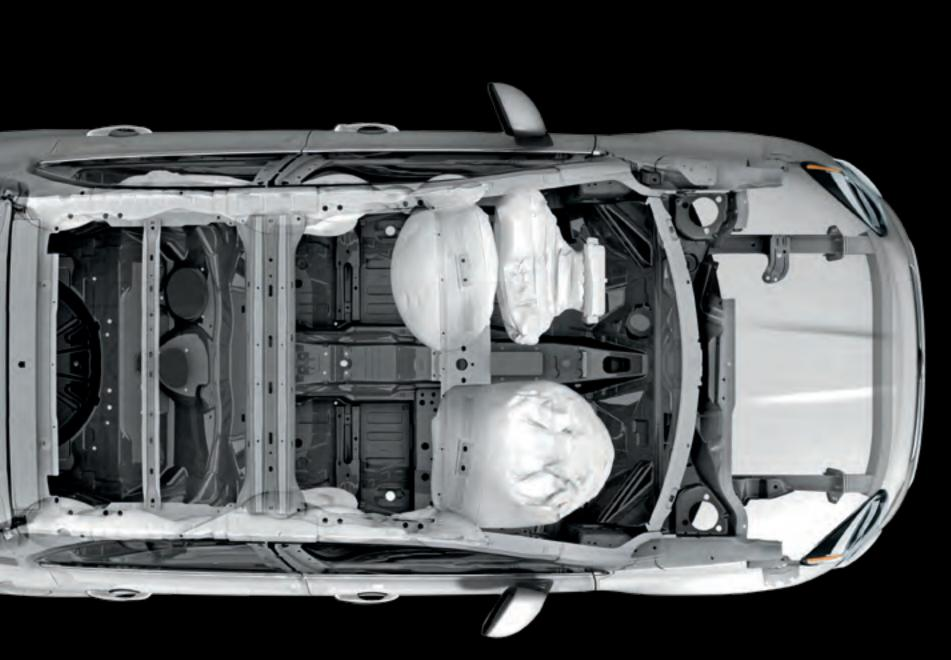
7 STANDARD AIR BAGS<sup>4</sup> Front-seat-mounted side, full-length side, driver's knee bolster and advanced multistage front air bags⁴ all work together, providing protection.
