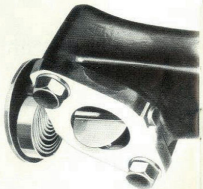
Manifold Heat Control, which is closed when motor is cold, automatically routes hot exhaust gases under carburetor until motor warms up.
