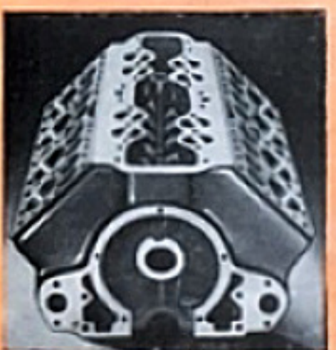
The V-type cylinder blocks and the upper part of the crankcase are cast in one piece. This design eliminates excess weight and gives longer life and better cooling. Cast alloy pistons give faster acceleration with slower wear.
