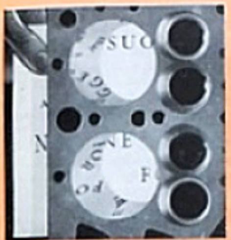
Cylinder walls are polished to a mirrorlike finish by two extra costly operations. This finish minimizes wear, seals compression and saves oil. It is another example of Ford precision methods.
