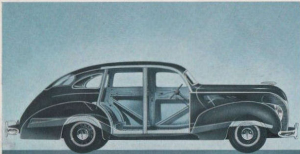
X-ray view of the Ford girder-type, all-steel body
