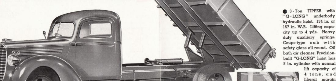
Coupe-type cab with bath air cleaner. Precisionbuilt "G-LONG" hoist has 8 in. cylinder with normal
