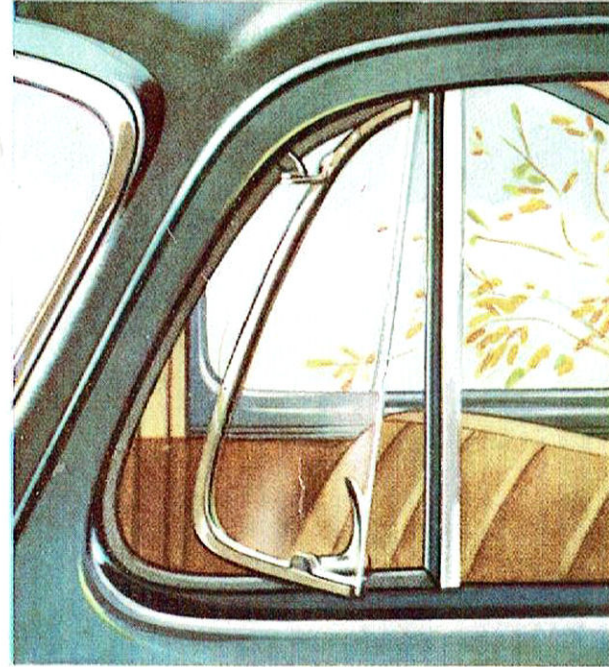
CONTROLLED VENTILATION. Draught-free ventilation is made possible by Prefect's adjustable quarter windows in front doors.
