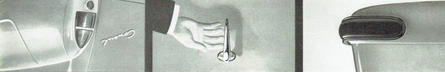
REAR END PROTECTION: Rubber-faced bumper-eyes curve right around the vital rear corners, absorb shocks better and do not show scratches.
