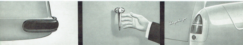
CENTRAL TAILGATE HANDLE allows easy, single-handed operation. The tailgate suspension chains are P.V.C. covered for load-protection.
