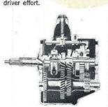
10. Heavy-duty 11" Clutch. Durable heavy-duty 11" clutch, with 123.7 sq. inch lining area, dissipates heat faster, for increased dependability and longer life. It combines with Ford's hydraulic clutch actuation for smooth, easy shifting, with less fatigue after a day's work.
