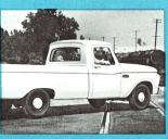
Twin I-Beam makes your 15 cwt. pick-up ride like a car. Low deflection-rate coil springs and large shock absorbers soak up jolts and vibra-The well appointed F 100 gains even greater cab comfort from Twin I-Beam.
