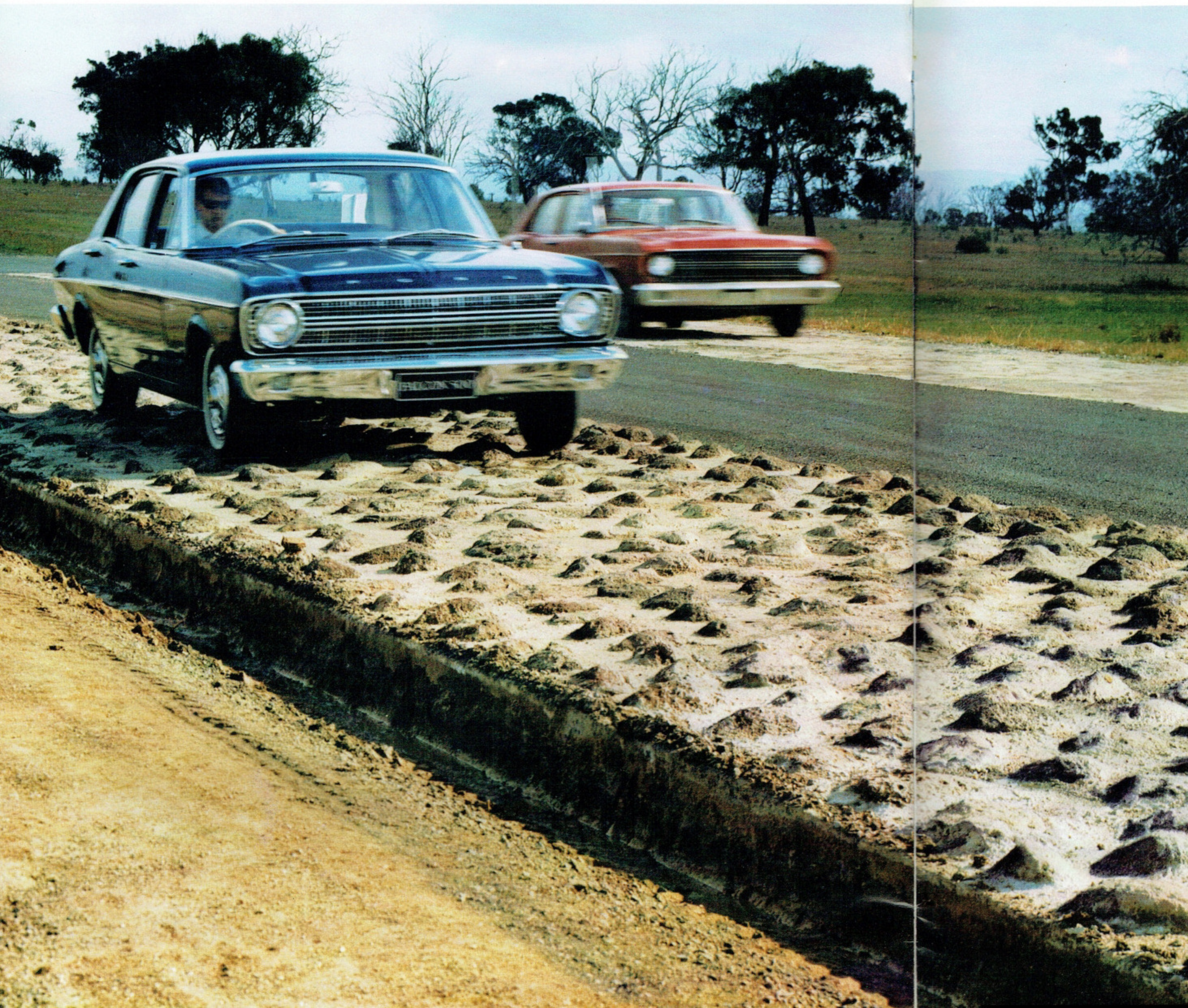
C-a-r---thumper! "Chuck Hole Road" contains man-made holes and bumps of every shape and size . . . varying depths and heights. As one wheel slams into a bump, the other thumps into a hole . . . inflicting bone-jarring jounce and rebound
