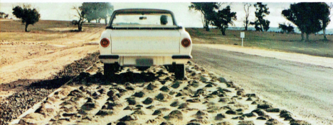
Above: "Cobblestone Road" — one of the "nightmare" stretches, tests durability of body structure, steering gear and linkage, suspension components and shock absorbers.
