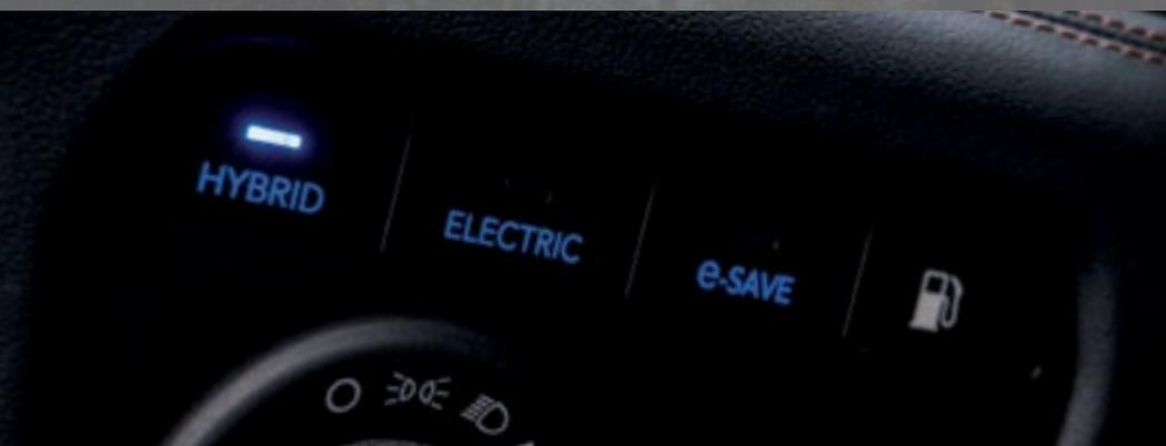
**YOU CHOOSE HOW AND WHEN TO OPTIMIZE THE HYBRID DRIVETRAIN** via push-button controls on the dashboard. Select HYBRID for the best of both worlds, ELECTRIC to only use battery power, or e-SAVE to reserve battery power for later — like for low-emission zones in cities or driving through a majestic cedar forest — where you'll enjoy near-silent exploring with maximum torque and horsepower.
