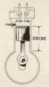
other is a stroke. Each revolution of the crankshaft is two strokes. Two revolutions of the crankshaft is one cycle of four strokes.
