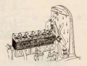
the water absorbing the heat and rejecting it to the air through the radiator.
