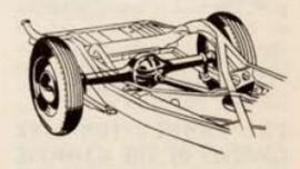
rear axle gears and axle shaft to the rear wheels. The power developed in the combustion chambers is thus utilized to move the car forward at the will of the driver.
