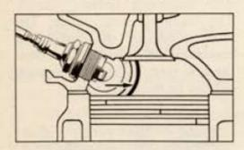
even a gentle breeze, the fire travels rapidly across the field. This is exactly what happens in the fiery combustion chamber. Scientists have photographed this action and have found that it takes about 1/350 of a second for the flame to travel from one side of the chamber to the other.
