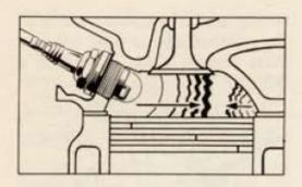
ing up a hill. It is objectionable because it is a disagreeable noise and it results in excessive heating and loss of power in the engine. During knock the last part of the charge burns almost instantaneously and is accompanied by a rapid rise in pressure. The total pressure on the piston head is raised in an instant by a thousand pounds.
