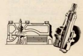
power strokes, when the mixture is compressed into the clearance space, ignition occurs.
