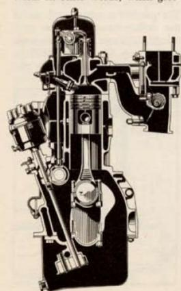
line is burned new products are formed, one of which is the power which pushes the piston downward. This downward movement of the piston is transformed into rotary motion by the crankshaft.
