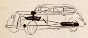
place the storage tank as far away from the workmen and factory as possible to eliminate the danger from fire. For the same reason, the raw product for the automobile is stored in a tank in the rear, away from the passengers and hot engine. The tank is kept cool by the air circulating around it and, in case of danger to the car, the passengers are not drenched in the highly inflammable gasoline.
