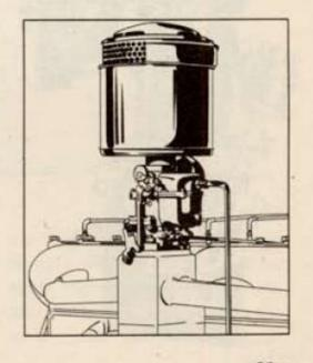
raw products are mixed in the right proportions. To keep the dust and dirt out of the engine, the air is usually passed through an air filter placed at the air entrance to the carburetor. An intake silencer, also located on the carburetor, eliminates the noise which issues from the air entrance at high speed.
