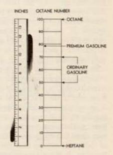
The octane numbers of gasolines for automobiles range from 50 to 78. Ethyl gasoline is held at a standard of 78 octane number all over the country.
