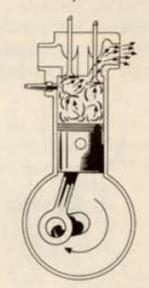
der to make room for a new charge. The exhaust valve opens and the piston, moving upward, forces the burned gases out through the exhaust port and exhaust manifold.
