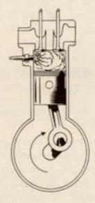
ignites the mixture. At once the cylinder pressure rises to over 400 pounds per square inch. The hot gases, expanding against the walls of the enclosed chamber, push the only movable part, the piston, downward. This movement is transferred to the crankshaft by the connecting rod.
