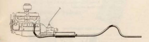
chamber we would hear a loud barking roar whenever the engine was in operation. To eliminate this noise, the gases are passed through a device called a muffler ing to you as indicating in some measure how all fields of science merge together in giving you the dependable service supplied by the modern motor car.
