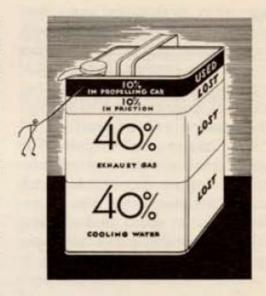
take care of these large quantities of heat. The cooling system absorbs 40 per cent of this waste and rejects it to the air.
