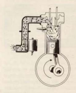
to give each cylinder its share of air and fuel. The manifold thus acts as the distributing system for the raw materials from the carburetor to the power chambers or cylinders.
