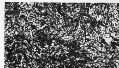
MICROGRAPH OF CORE OF CASE HARDENED STEEL MAGNIFIED 500 DIAMETERS
