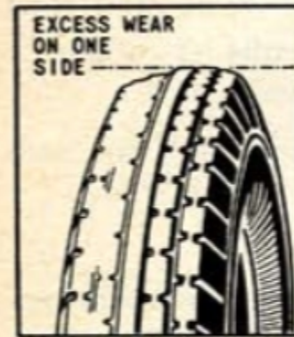
WEAR DUE TO CAMBER
