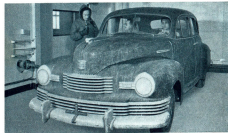
Completely equipped laboratories duplicate the most difficult operating conditions. Here engineers are testing cold-weather operation in temperatures 40° below zero.
