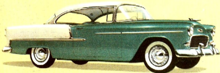
1955 CHEVROLET BEL AIR SPORT COUPE: For 1955 Chevrolet offers two separate series of cars, one equipped with the popular Chevrolet six-cylinder in-line engine, and one powered by the brand-new Turbo-Fire V-8, high-compression engine. Powerglide transmission is available on both. Wheelbase for both series is 115 inches. All Chevrolet cars for 1955 feature GM's panoramic windshield.
