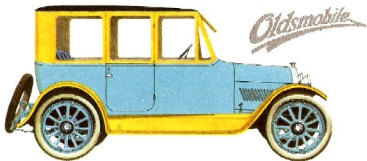
1919 OLDSMOBILE SEDAN: (Representing GM's 1,000,000th Car) Powered by a six-cylinder, 45-horsepower engine, it got 13 miles to the gallon of gasoline. Wheelbase was 112 inches. The slanted windshield was years before its time.
