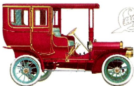
1908 CADILLAC "MODEL G" LIMOUSINE: One of the earliest enclosed cars produced by Cadillac, this model had a four-cylinder, 25-horsepower engine, and a top speed of 50 miles per hour. Wheelbase was 100 inches.
