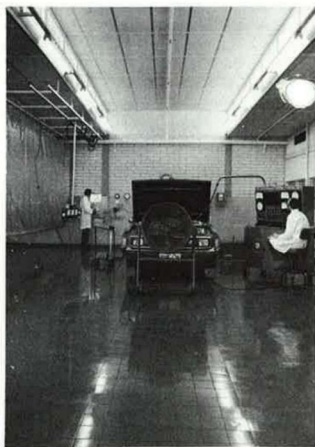
Testing exhaust emissions at Chrysler's Lonsdale engine factory.
