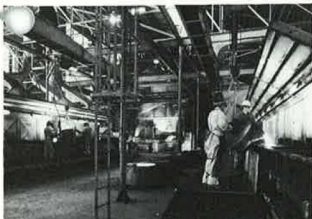
Pouring molten iron into engine moulds
