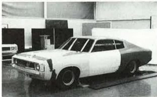
Building up a clay model Charger prototype in clay
