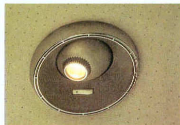
Rear compartment reading lamps.
