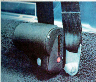
Retractable vehicle-sensitive seat belts.
