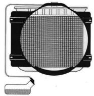
It includes a seven blade fan which increases the air flow through the larger capacity radiator. The shroud directs the airstream through the core. And the coolant recovery system eliminates topping up.
