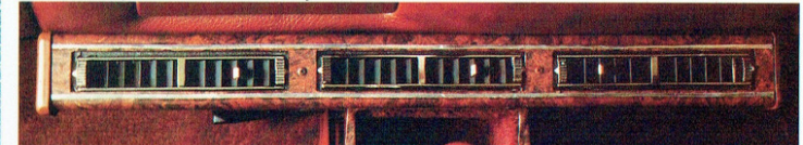
Full width air-conditioning vents.
