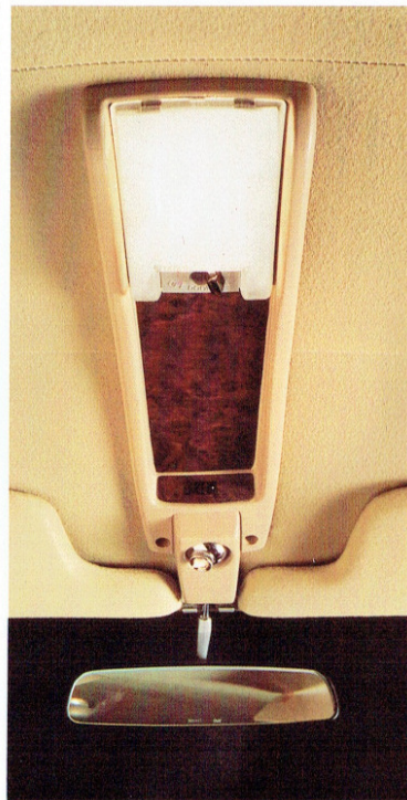
Roof console containing dome lamp and eyeball navigation light.
