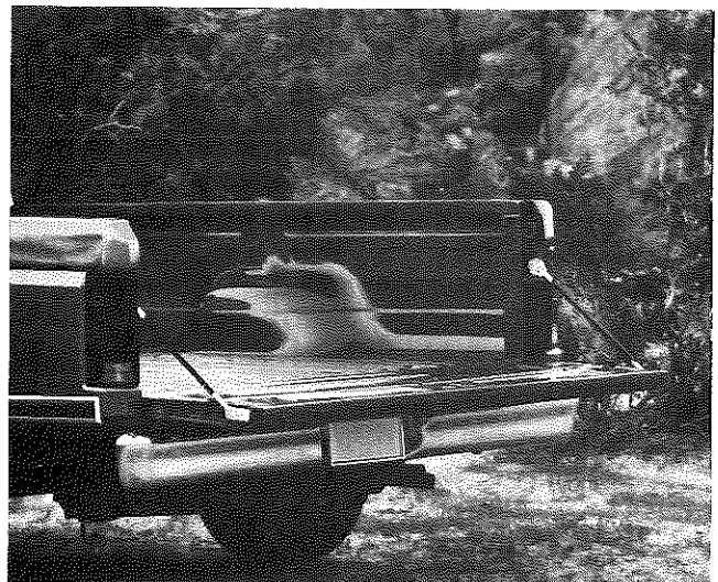
Easily Disconnected Support Cables and Special Hinges Provide for Easy Removal of Tailgate
