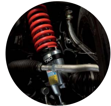
TRD Pro Bilstein® shocks with remote reservoirs
