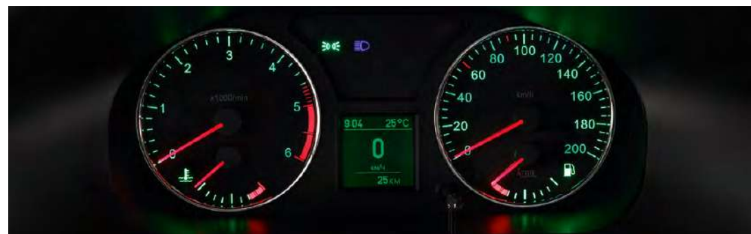
New instrument cluster with trip computer and temperature gauge
