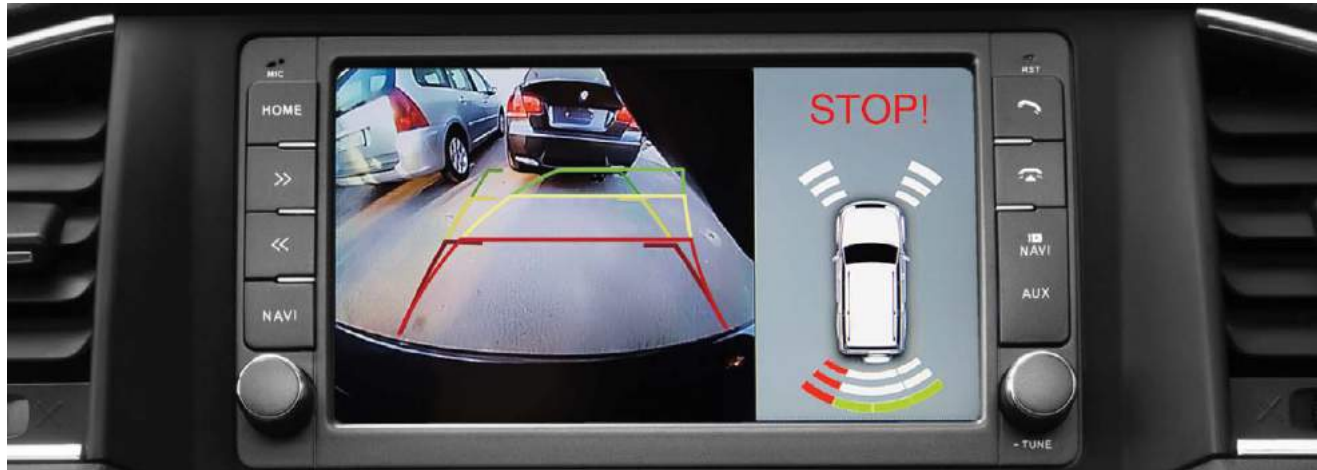
When backing up a vehicle, a color display shows the view from the rear camera with dynamic indexing lines, and front and rear parking sensor signals
