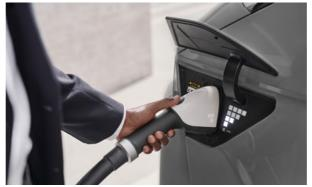
In just 18 minutes, you can top up from a 10% to an 80% charge with a 350 kW DC fast charger
