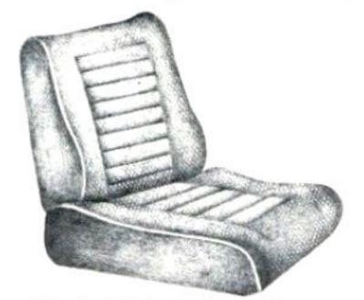
with built-in twin coil springs and an hydraulic shock absorber let you take it easy.
