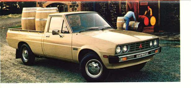
EXPRESS ONE TONNE UTILITY. Takes giant loads of up to 1000 kg. Outback there's strong, ribbed steel cargo deck with easy loading drop down tail-gate. Upfront there's plenty of room for a driver and 2 passengers. And the specially designed bench seat gives ideal back support. Under the bonnet there's a reliable and economical 1.6 litre Saturn Engine. And power assisted front disc brakes give safe, sure stopping over all types of terrain.
