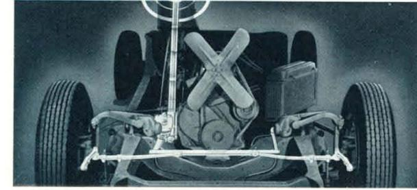
One of the reasons why you can drive far in Oldsmobile and at the end feel rested is DUAL CENTRE-CONTROL STEERING. No road shocks are transmitted to the steering wheel, neither do the wheels ever "fight" the driver. Finger pressure is sufficient for steering. The wheels centre themselves automatically,
