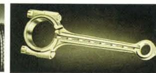
RODS, redesigned for greater strength, (coil springs at all 4 wheels) gives a retain the famous Oldsmobile characteristic "gliding ride". Double action hydraulic - rifle-drilled, they carry oil under pressure to piston rings and cylinder walls.
