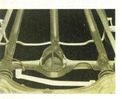
4 - WAY STABILIZA-TION enhances Oldsmobile's wonderful steadiness. At the left are seen the stabilizer arms extending from rear axle to frame, which do not allow any fore-and-aft pitching, and the rugged rear stabilizer which, with the front-end stabilizer, control rolling motion and prevent body sway.
