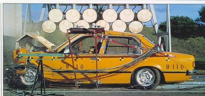
Left: Commodore's front body absorbs impact forces. The engine hood folds backward rather than penetrating the windscreen. Barrier impact testing under lights and cameras proves Commodore's passenger protection.
