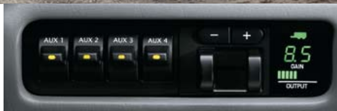
Trailer Brake Controller shown to the right of Upfitter Switches, which are standard on F-350/F-450/F-550 Chassis Cab; optional on F-250/F-350 Pickup (66S).
