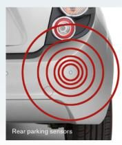
The CDX eases into and out of tight parking spaces, thanks to its rear parking sensors. Audible warnings indicate the proximity of potential obstacles.
