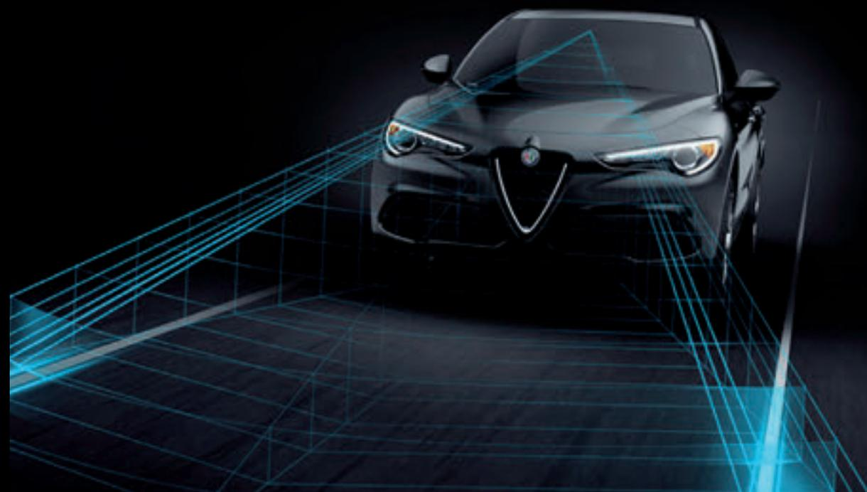
**HILL START ASSIST (HSA) AND HILL DESCENT CONTROL (HDC)** These standard systems aid the driver during manoeuvres when the vehicle is on a slope. HSA maintains and releases brake pressure during vehicle drive-off, while HDC maintains a constant speed by varying brake pressure, allowing a controlled vehicle descent.
