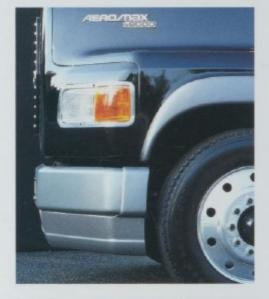
Aero headlights with integral flush turn signal for improved aerodynamic air flow around the fenders.
