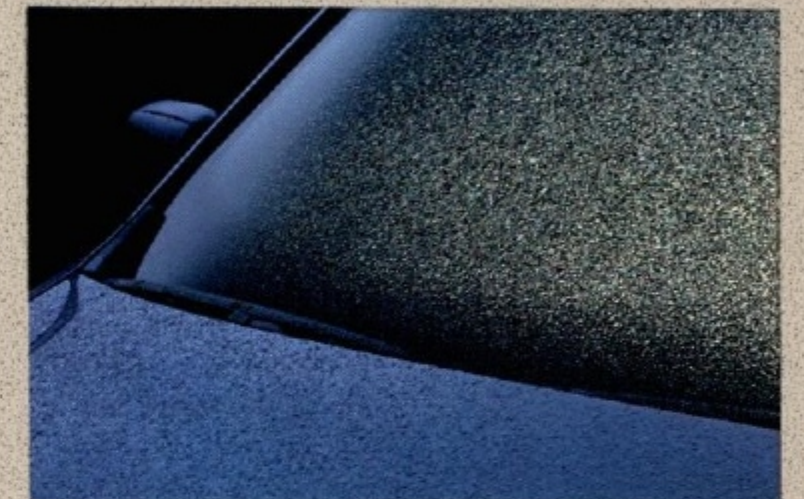
Continental's optional Insta-Clear® windshield uses a transparent metallic coating to spread heat over the windshield's entire surface.
