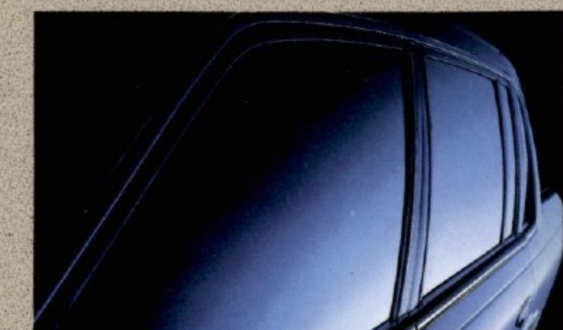
Flush-mounted glass reduces aerodynamic drag.
