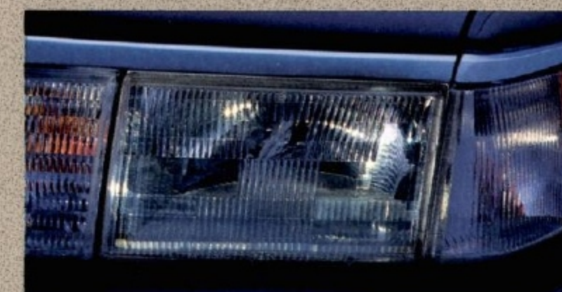
Aerodynamic headlamps have impact-resistant polycarbonate lenses.
