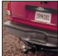
A Class III trailer hitch. The ball-mount must be purchased separately.
