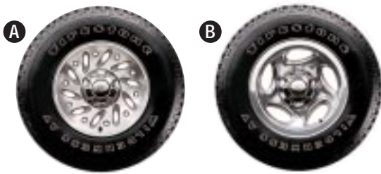
A 15" deep-dish cast aluminum wheel (standard) B 16" machined aluminum wheel (included in Premium Sport Group option)
