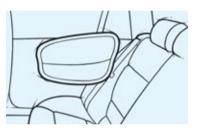
Rear side airbags protect your upper body in a side-on collision; the side airbag significantly reduces the risk of injury at pelvic and chest level.
