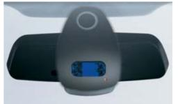
☐ Rain sensor uses an infrared light to measure the amount of rain. When the wipers are in the "intermittent" mode, the rain sensor automatically adjusts the windshield wiping interval as needed. (Standard on the 540i.)
