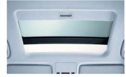
■ Glass sunroof allows natural light to enter the cabin. For convenience, it has a one-touch open and close feature with anti-trapping, as well as a tilt function for ventilating the inside of your car on hot summer days.
