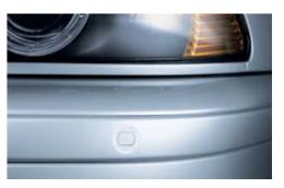
□ Park Distance Control (PDC) uses ultrasonic sensors in the front and rear bumpers to help you judge the distance to other cars and unseen objects when parking. The beeping becomes faster as your bumper approaches the object, turning into a constant tone when the distance is less than 30 centimetres.
