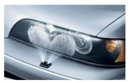
☐ Heated headlight washers help keep lights clean of ice, mud, road salt and other coatings, for maximum road lighting and enhanced driving safety. (Standard on the 540i.)
