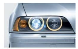
■ Xenon headlights illuminate the road ahead ■ Dynamic Stability Control (DSC III) recognizes and to the side with brilliant clarity. These head- the risk of the car skidding very early and stabilizes lights also feature auto-levelling to adjust for the car within milliseconds. varying passenger and cargo loads.
