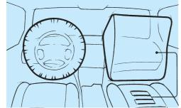
■ Driver and front passenger airbags protect your head and upper body in a frontal collision from hitting the steering wheel or instrument panel; depending on the severity of the impact, the airbags are inflated via a two-stage gas generator (impact-depending system); the front passenger airbag comes complete with a seat occupancy detector.
