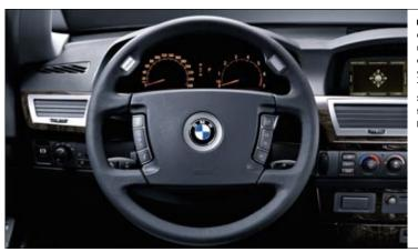
■ Multi-function steering wheel for very comfortable and convenient operation of numerous functions without taking your eyes off of the road – and without taking your hands off the steering wheel. Telephone functions, radio adjustment, STEPTRONIC, as well as many other functions are accessible through the buttons on the steering wheel.
