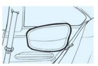
☐ **Rear side airbags** protect your thorax in a side-on collision; the side airbag significantly reduces the risk of injury at pelvic and chest level.
