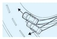
■ Dynamic Stability Control (DSC) recognizes the risk of the car skidding very early and stabilizes the car within milliseconds. Also includes Dynamic Brake Control (DBC).
