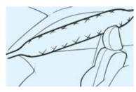
■ ITS Head Protection System (HPS) for the driver and front passenger provides effective protection of your head and upper body in a collision from the side.
