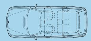
\* Head room measurement with sunroof is 940 mm. All dimensions in millimetres. Figures in [] apply to All-wheel drive. Luggage compartment capacity 435-1617 litres (15.2-47.1 cu ft) (to VDA standard). Turning Circle 10.5 m on 325i, 10.9 m on 325xi
