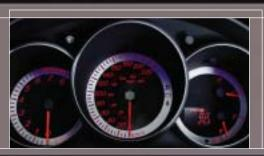
GLOWING REPORT. Tri-mode electro luminescent gauges, standard on the Mazda 3 GT and Mazda 3 Sport models, display three distinct colour combinations depending on whether it's daytime, night-time or the ignition is off.
