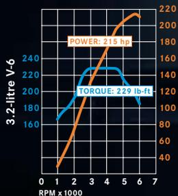
Smoothness and flexibility merge seamlessly in the CLK320's 215-hp 3.2-litre V-6. But the real magic lies in its incredibly broad, flat torque curve that brings a heady 229 lb-ft of peak force from 3,000 to 4,600 rpm. It makes a CLK320 remarkably quick off the line and helps it hit 100 km/h in as little as 7.6 seconds.<sup>1</sup>
