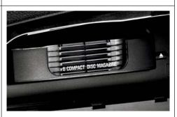
$\Box$  **CD Changer,** for six CDs, integrated into the back of the glovebox.
