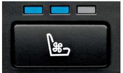
□ **Ventilated seats** for the driver and front passenger. Ventilator fans are built into the outside seats and blow air upwards through an internal web and the micro-perforated Nasca Leather to provide active ventilation.
