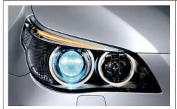
■ Xenon headlights illuminate the road ahead and to the side with brilliant clarity. These headlights also feature auto-levelling to adjust for varying passenger and cargo loads. In conjunction with the new Adapative Headlights (optional on the 530i), this also means much improved visibility in bends, as the adjustable headlights are directed into the bend as soon as the vehicle begins cornering.
