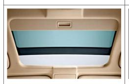
■ Glass sunroof allows natural light to enter the cabin. For convenience, it has a "one touch" open-and-close feature with anti-trapping, as well as a tilt function for ventilating the inside of your car on hot summer days.
