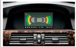
☐ Park Distance Control (PDC) uses ultrasonic sensors in the bumpers to help you judge the distance to other cars and unseen objects when parking. The beeping becomes faster as your bumper approaches the object, turning into a constant tone when the distance is less than 30 centimetres.
