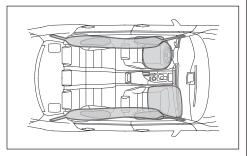
■ Airbag system: In the event of a collision, only the airbags that are needed are deployed. Up to eight airbags offer specific protection: the driver and front passenger airbags (which are released at different speeds, depending on the strength of the impact), the front-to-rear head airbags, the side airbags in the front and the optional side airbags at the rear.
