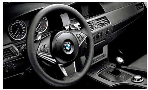
☐ Sequential Manual Gearbox (SMG®) offers both normal and sport manual transmission modes via the paddles on the steering wheel or the shifter. The sport mode may be selected by depressing the "sport" button. (European model shown.)
