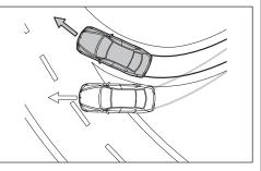
■ Dynamic Stability Control (DSC) including Dynamic Traction Control (DTC), Cornering Brake Control (CBC) and Dynamic Brake Control (DBC). DSC recognizes the risk of swerving from the start and stabilizes the car within milliseconds. DTC is a subsidiary function of DSC and permits increased wheel slip within defined limits, in order to maximize propulsion in specific situations.
