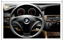
■ Multi-function leather steering wheel allows for convenient operation of numerous functions without being distracted from road traffic - which means you keep your hands on the wheel all the time. Buttons are included for audio, cruise control and telephone. Functionality of two separate buttons may be defined by the user.
