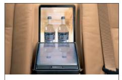
□ Cooling box, included with the rear air conditioning system, is accessible when the centre armrest is folded down, and provides capacity for one or two suitable drink bottles and some snacks. (Available only on the 745Li and 760Li.)
