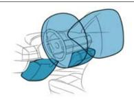
■ Active knee protection is an advanced unique new safety feature. Located in the lower dashboard, it is activated in a frontal crash, adding further protection to the restraint system for front seat occupants.
