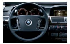
■ Multi-function steering wheel offers convenient operation of numerous functions without taking your eyes off of the road oryour hands off the steering wheel. Telephone functions, radio adjustment and STEPTRONIC, as well as many other functions, are accessible through the buttons on the steering wheel.
