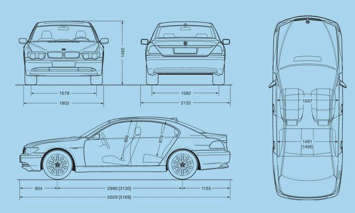
All dimensions of drawings in millimetres. Figures in [] apply to the 745Li and 760Li. 745i, 745Li, 760Li Luggage Compartment Capacity 500 litres.
