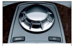
■ The Controller serves as the principal iDrive entry unit. Operating this rotary / push button intuitively with just one hand, you can activate and mastermind numerous functions via the Control Display. Menu guidance is oriented following the four directions of the compass, with four submenus to choose from: Climate, Communications, Navigation and Entertainment.
