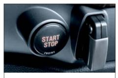
■ Start/Stop button for starting the car together with the remote control. Drivers insert the remote control into the starter switch until it rests in position. After receiving authorization, they can start/stop their BMW simply by pressing a button.
