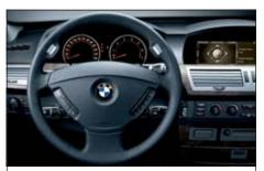
□ Sport leather steering wheel with three spokes offers a sporty design for perfect handling and control. Buttons are integrated for STEPTRONIC and radio, as well as the telephone, voice and audio control. (Available only on the 745i and 745Li with Sport Package.)
