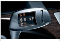
■ Six-speed automatic transmission with electronic gearshift and STEPTRONIC. You operate the transmission via the switch on the steering column or the STEPTRONIC buttons on the steering wheel. Electric shiftby-wire transmission allows a very quick and absolutely faultless shift of gears in the interest of supreme driving dynamics.
