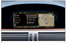
■ Navigation System presents information in the dazzle-free Control Display, including the BMW Professional radio. Driving information is provided by the voice computer, with further data added by the direction arrow (on the Info display) or map.
