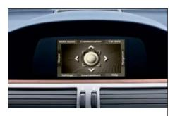
■ Control Display in LCD technology with screen. Using the Controller, you can present all functions masterminded by iDrive on the Control Display – for example, route information or other items such as the radio program or information from the on-board computer.
