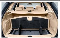
□ Storage compartment package for a practical and even more versatile luggage compartment. This equipment package includes an underfloor storage space with adjustable compartments, as well as two foldable dividers for securing objects of different sizes. Also included: straps on the side walls, multi-purpose holders and a net on the left-hand side for smaller items.
