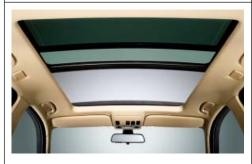
■ Panorama glass roof with large opening/ transparent area and speed-dependent wind deflector. Both glass sections can be angled by pressing a button. The front section can also be used as a sliding roof and comes with an electric sunblind, comfort opening/closing function and trap release.
