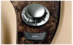
■ Controller, the central iDrive control element (for use by driver and front passenger). This turn/press button enables intuitive control of a variety of functions shown on the Control Display. The menu system is based on the four compass directions and provides a choice of four individual menus: climate, communication, navigation and entertainment.
