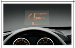
☐ **Head-Up Display** shows the driver relevant information, such as the current speed. Other display data include direction arrows from the navigation system, Active Cruise Control functions and Check/Control data.
