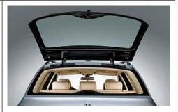
■ Rear window, with separate opening function: can be opened separately for quick and easy loading and unloading of objects.
