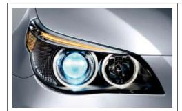
■ Xenon headlights illuminate the road ahead and to the side with brilliant clarity. These headlights also feature auto-levelling to adjust for varying passenger and cargo loads. In conjunction with Adaptive Headlights, this also means much improved visibility in bends, as the adjustable headlights are directed into the bend as soon as the vehicle begins cornering.
