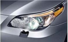
■ Headlight cleaning system ensures optimum headlight brightness in all kinds of weather. When the lights are on, the headlights are automatically cleaned in parallel with the windscreen.
