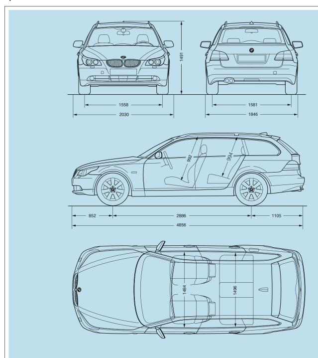
All dimensions in millimetres. Luggage compartment capacity (as per VDA standard):  $500\!-\!1650\,litres$  (17.7–58.3 cu ft).
